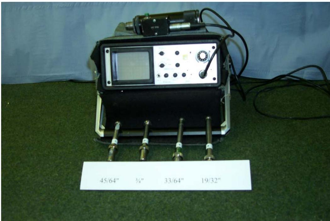
Figure C-3: A Photograph of the Rohmann Rototest Instrument.
