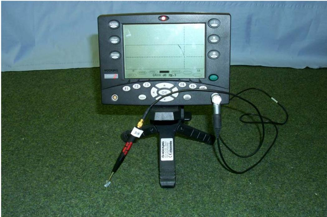
Figure C-2: A Photograph of the Hocking Locator 2 Instrument.
