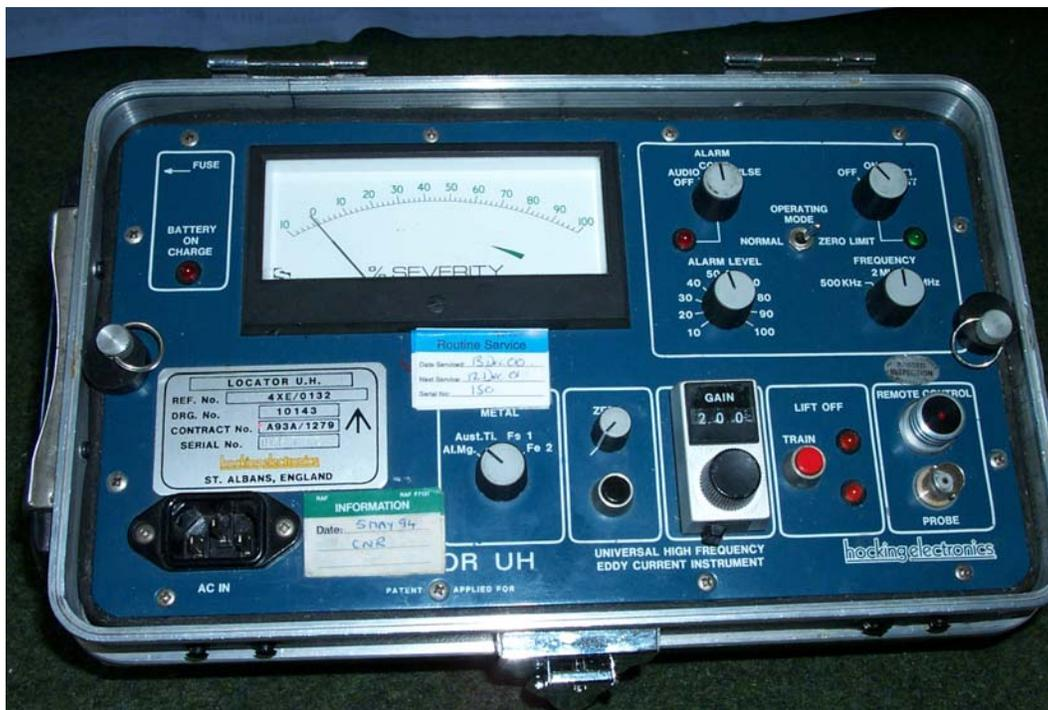
Figure C-1: A Photograph of the Hocking Locator UH Instrument.
